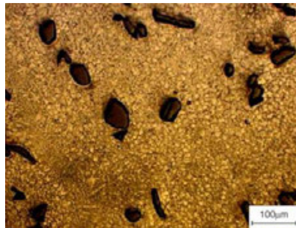
Figure 24. Central zone of the surface layer of the MCMgAl6Zn1 alloy after SiC powder alloying, laser power 2.0 kW, laser scan rate 0.50 m/min
