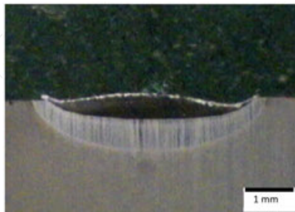
Figure 11. 32CrMoV12-28 steel alloyed with VC powder, laser power 1.2 kW
