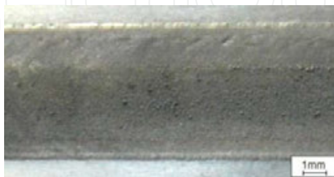
Figure 19. Surface layer of the MCMgAl9Zn1 alloy after WC powder feeding, laser power 2.0 kW, laser scan rate 0.5 m/min
