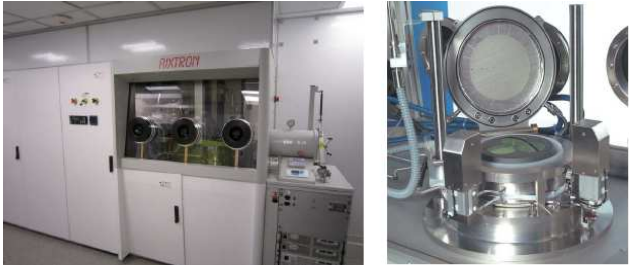
Figure 14. Photograph of New-generation AIXTRON CCS 3x2 " high temperature III-Nitride 3x2 MOCVD growth Chamber open for loading wafers showing close-coupled showerhead [26]
