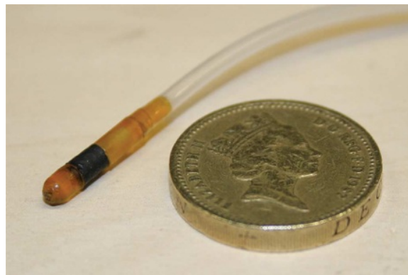
Figure 11. Ablation catheter with force sensor (Reference [29]). The outer diameter is 3mm (9Fr in French scale which is used to express size of catheters).
