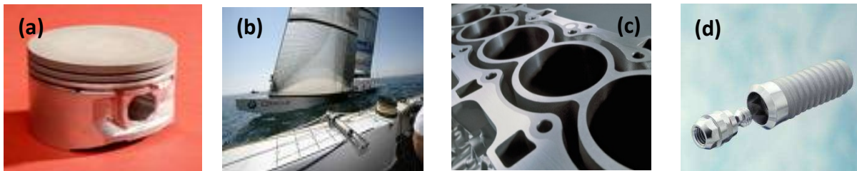
Figure 5. Use of PEO coatings on: (a) engine piston, (b) racing yachts, (c) engine block and (d) dental implants.
