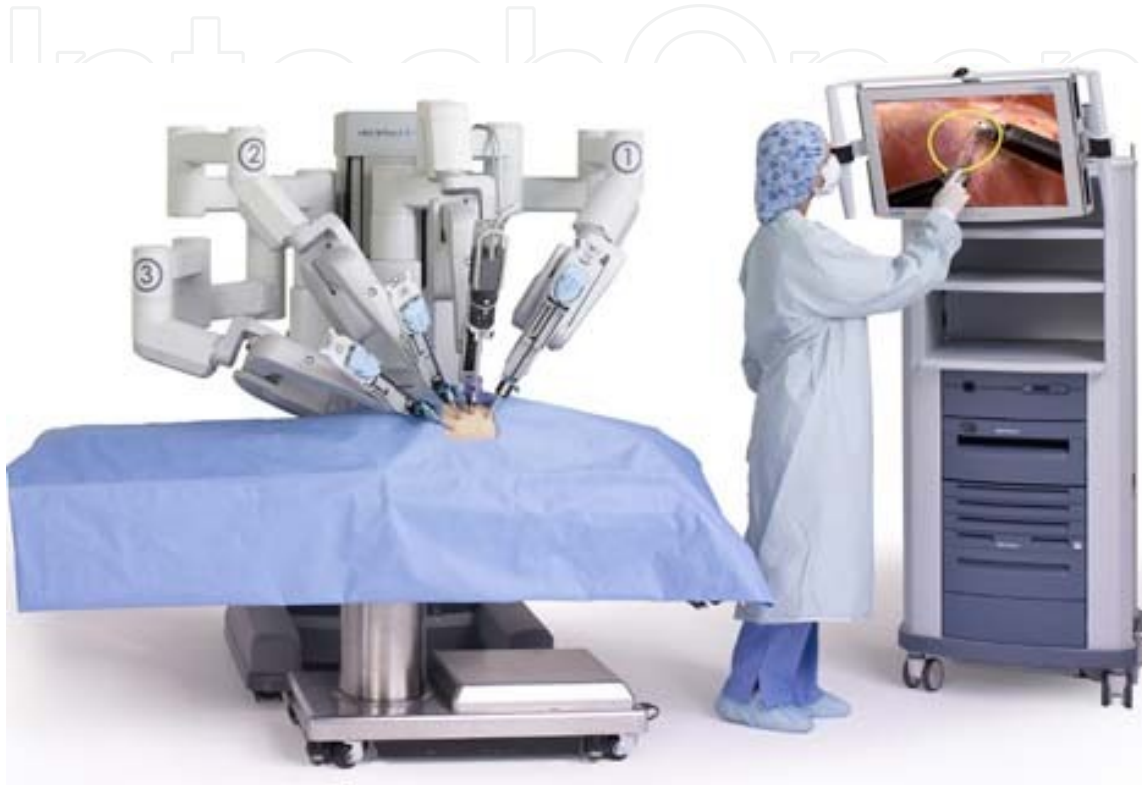
Figure 1. [25]: showing the robotic stack/cart and the monitor used by the assistant to follow the operation
