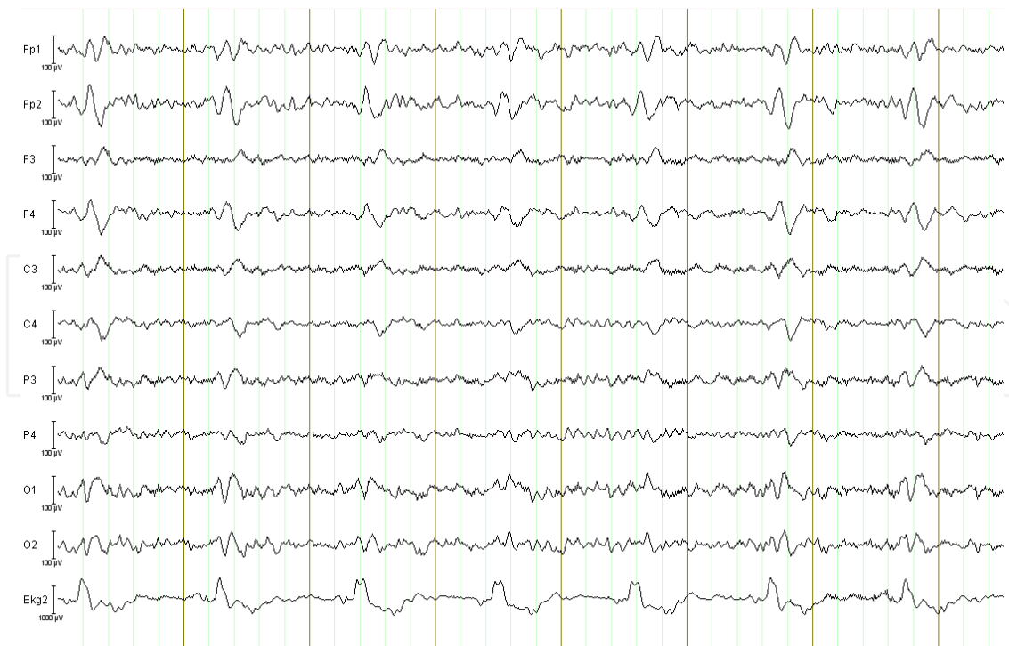
Figure 3. Shows ECG and EEG signals measured inside an MRI scanner without applying the imaging gradients. The BCG artefacts are embedded in each channel.
