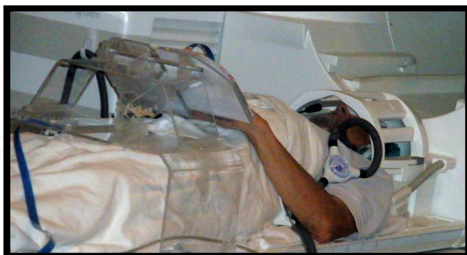
Figure 5. A subject on the scanner bed operating our novel multimodal MRI-compatible drawing device. The plexiglass gantry supports a drawing tablet while a fiber-optic drawing stylus captures and records the drawing movements with high precision. This motion-capture information synchronized with the fMRI signal allows the effect of behavioral events during drawing to be correlated with brain activation.
