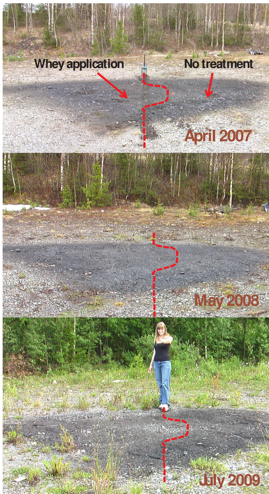
Figure 11. One time treatment of left part of oil spot with 200 l fresh milk whey.
