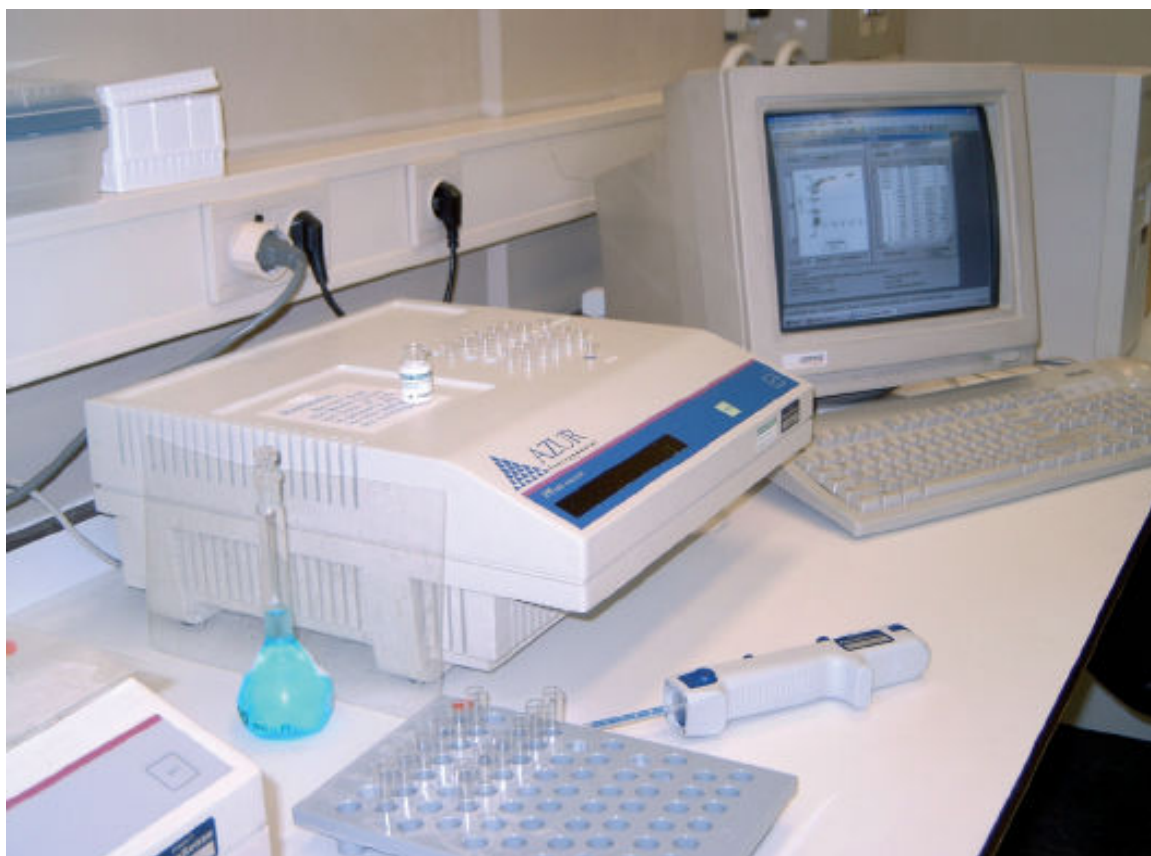
Figure 5. Equipment for measuring luminescence of Vibrio fischeri [94]
