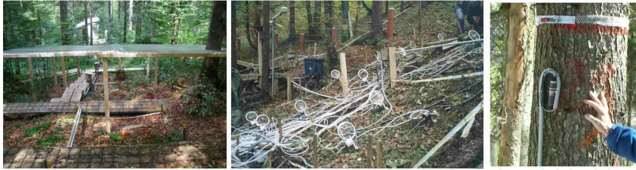
Figure 11. Elements of climate manipulation experiments. Roofs under the tree canopy enable the creation of artificial drought conditions (left), automatic chambers allows the continuous measurement of greenhouse-gas emissions from soils (center), stem diameter growth is a common response variable for the quantification of climate change effects (right).
