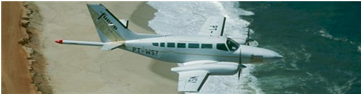
Figure 6. Fugro Airborne Surveys photo showing a magnetometer in a 'stinger' behind the fixed-wing aircraft.
