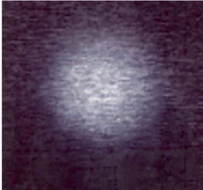
Figure 11. Response of an optical antenna located on the image of a blackbody radiator at 1000°K. This image was obtained by a relay optical system fabricated in ZnSe and having an F/# equal to 1 [29].
