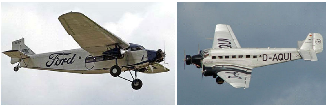
Figure 1. Airplanes with the skin made of corrugated sheet metal: Ford Trimotor (left) and Junkers Ju-52 (right)
