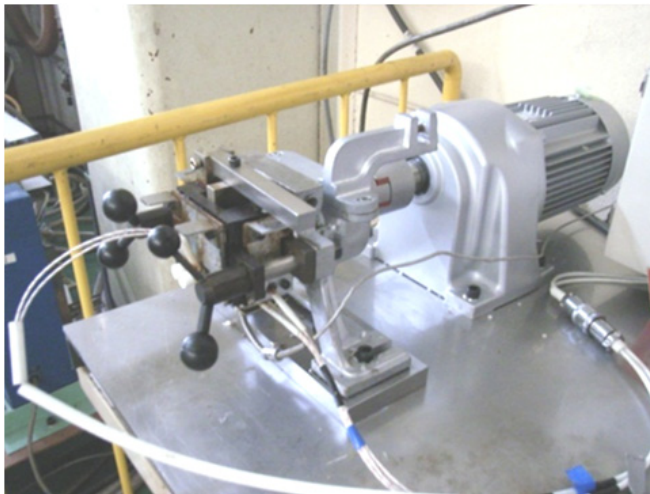
Figure 16. The small size mixer used for kneading the pellets with liquid paraffin.
