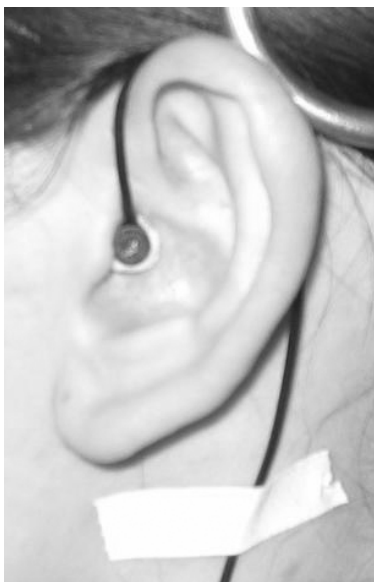
Figure 3. Blocked-ear-canal measurement with miniature microphone
