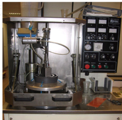
Figure 13. SOMOS lapping/polishing machine.
