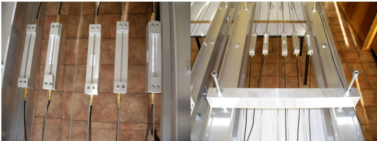
Figure 44. SAW-comprising vibration sensors attached to steel ropes
