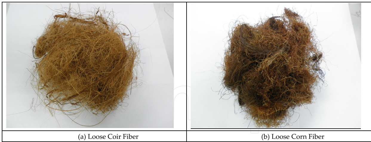
Figure 1. Loose forms (a) Coir Fiber (b) Corn Fiber
