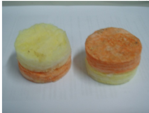
Figure 15. Double-layered 0.42pcf (yellow)/1.0pcf (orange), 1.75 cm thick each.
