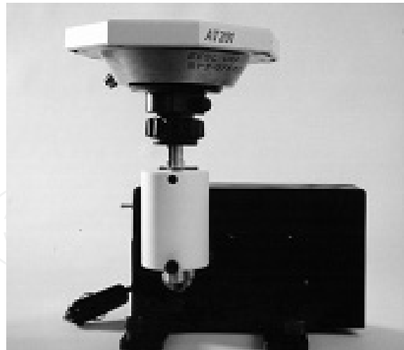
Figure 7. GPS antenna over the electro-mechanical oscillator
