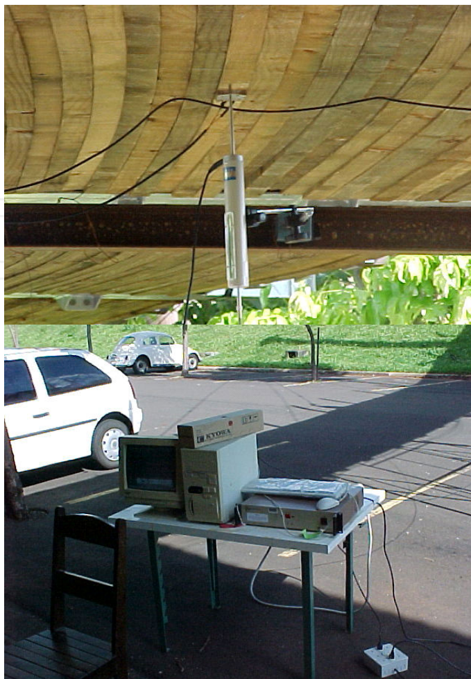
Figure 14. Transducer of displacements and data acquisition system
