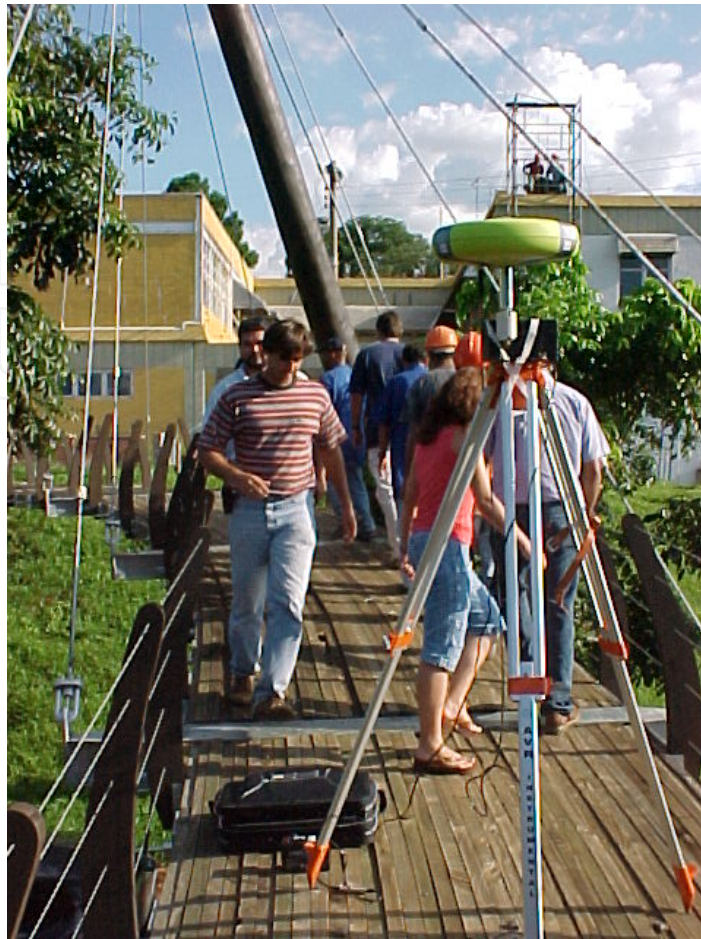
Figure 15. Front view of pedestrians walking on a footbridge and view of GPS antenna over oscillator
