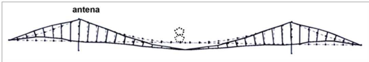
Figure 4. GPS mobile antennas under oscillations of the middle span of a bridge
