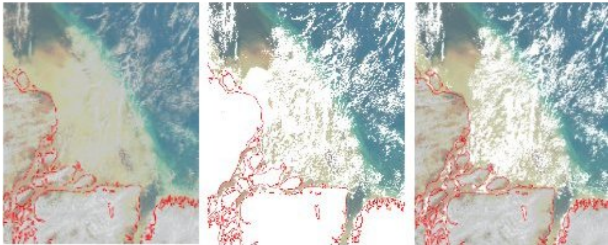
Figure 10. A color composite SeaWiFS image recorded over the Amazon delta area with no cloud mask (left), and after the application of the standard SeaWiFS NIR threshold (middle), and Nordkvist et al. [88] algorithm (right). The gain of clear water pixels is clearly seen when the latter algorithm is used instead of the standard SeaWiFS algorithm.
