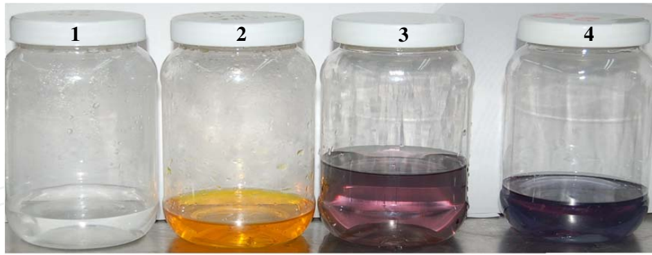
Figure 12. Chromium (VI) Reduction by lactic acid. 1. - Lactic acid standard solution (85%) 2. - Chromium (VI) standard solution (1.0 g /L). pH= 1.0 3.-100 mg Cr (VI)/L with lactic acid (100 mL) 4. - 1000 mg Cr (VI)/L with lactic acid (100 mL)
