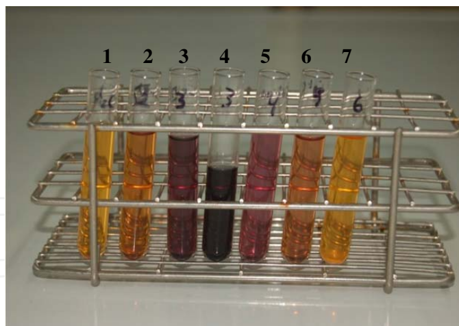
Figure 6. Cromazurol S Reaction 1.-Trideionized water pH=1.0 2.- K_2CrO_4 (50 \mu\text{g}/\text{mL} ) 3.- Cr(NO_3)_3 \cdot 9H_2O . (50 \mu\text{g}/\text{mL} ) 4.- Cr(NO_3)_3 \cdot 9H_2O . (500 \mu\text{g}/\text{mL} ) 5.- Problem (50 \mu\text{g}/\text{mL} ) 6.- Vitamin C (50 \mu\text{g}/\text{mL} ) 7.- Al_2(SO_4)_3 (50 \mu\text{g}/\text{mL} )
