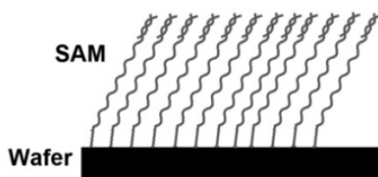
Figure 3. Schematic representation of a self assembled surface mono layer (SAM) resist. In this case linear resist molecules have made an arranged coating on the wafer.
