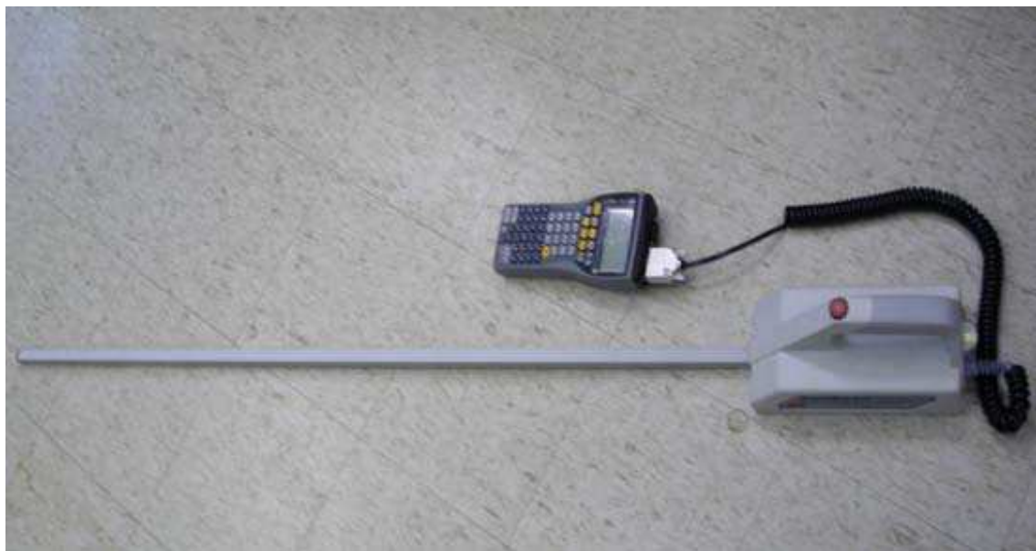
Figure 4. SunScan (Delta-T) canopy analyser for LAI and crop height measurements
