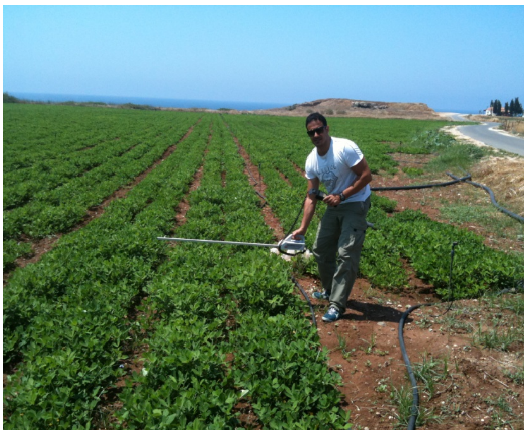
Figure 5. Use of SunScan canopy analyzer for LAI measurements (Papadavid, 2012)
