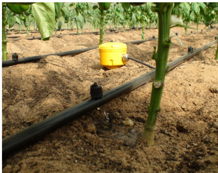
Figure 6. wireless sensor in the field that detects soil water status at various depths.
