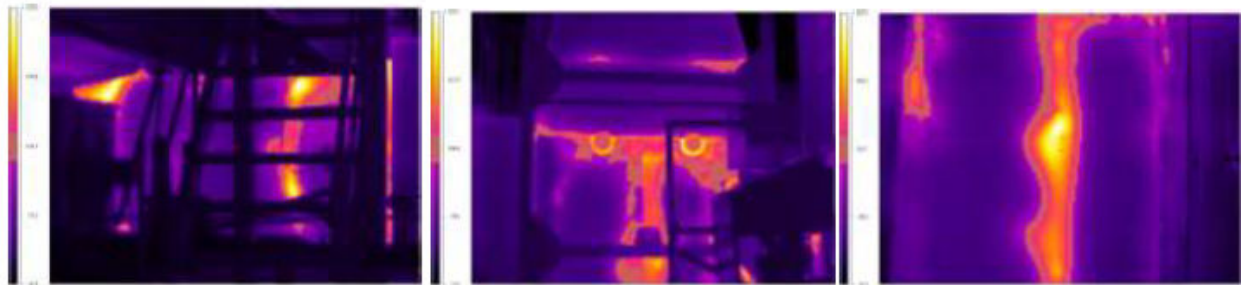
Figure 17. Temperature isotherms, in infrared, in the channel connecting the gas turbine and the afterburning installation (silencer – by-pass assembly – connecting transom)
