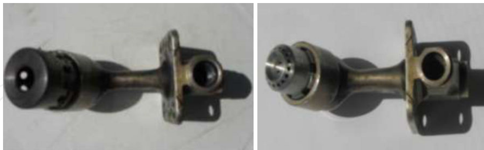
Figure 9. Injectors for liquid fuel for TV2-117A (left) and landfill gas for TA2 bio (right) [2]
