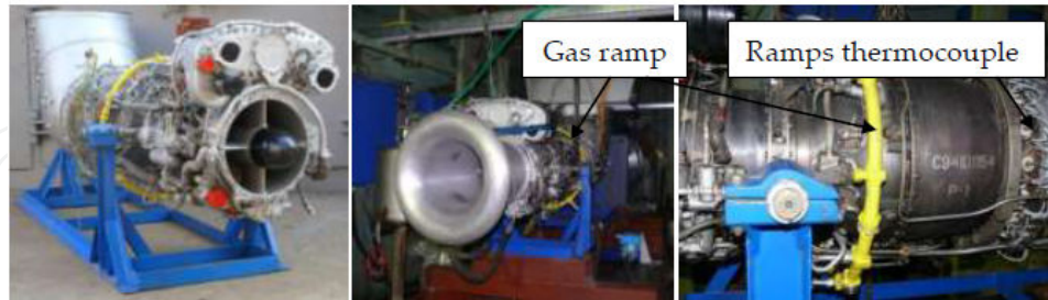
Figure 10. TA2 gas turbine (left) and TA2 bio gas turbine in the test cell (centre, right)
