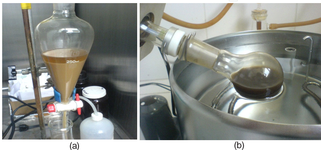
Figure 1. a) Emulsification of hydrocarbons. (b) Oil recovery.
