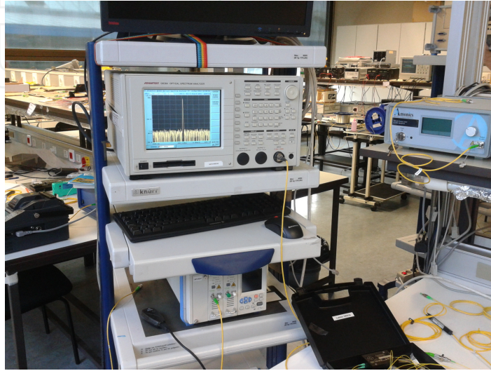
Figure 2. Experimental setup of a short-cavity fiber laser
