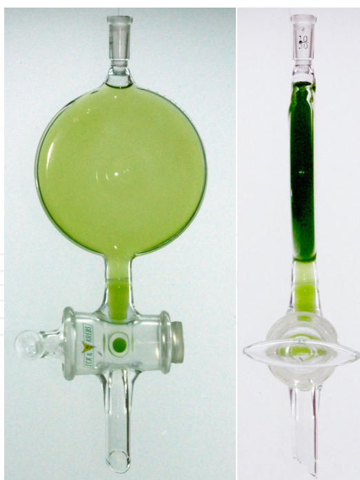
Figure 13. The “lollipop” is a laboratory apparatus for the purpose of cultivating algae to track the path of ^{14}\text{CO}_2 . This first glass photobioreactor was designed by Andrew A. Benson and is exhibited to the left in face view, filled with Haematococcus thermalis . The large 4 mm bore of the stopcock is featured by fill with the green alga. Viewed from the side, right, the characteristic thin layer of the algal culture is revealed.
