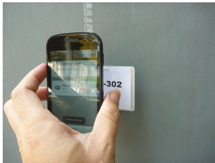
Figure 2. displayed the RFID-enabled smartphone with NFC technology and HF RFID tags using in the study.
