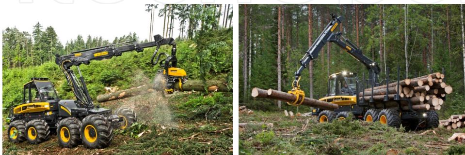
Figure 3. Examples of a harvester and a forwarder [1].
