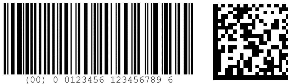
Figure 5. Examples of a GS1-128 code and GS1 DataMatrix [4].
