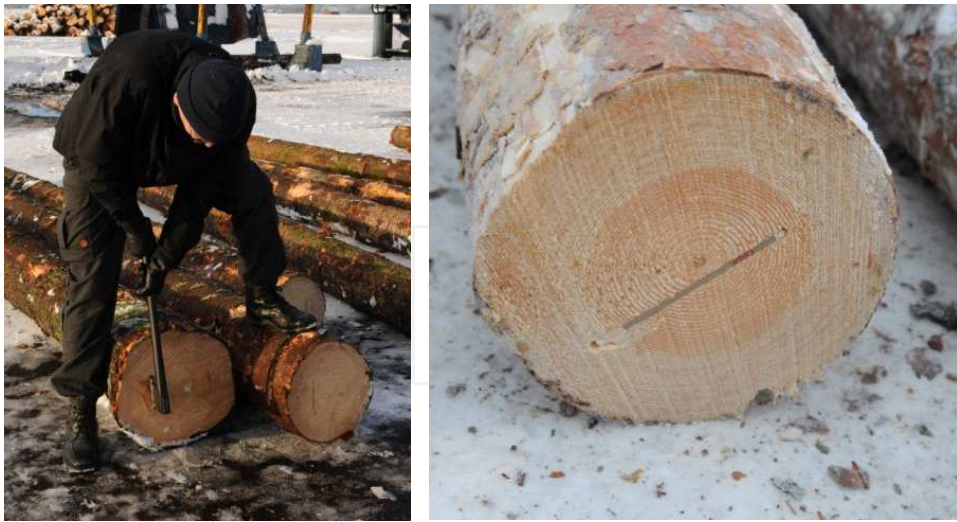
Figure 9. Application of the tag and the tag inserted into the end of the log.
