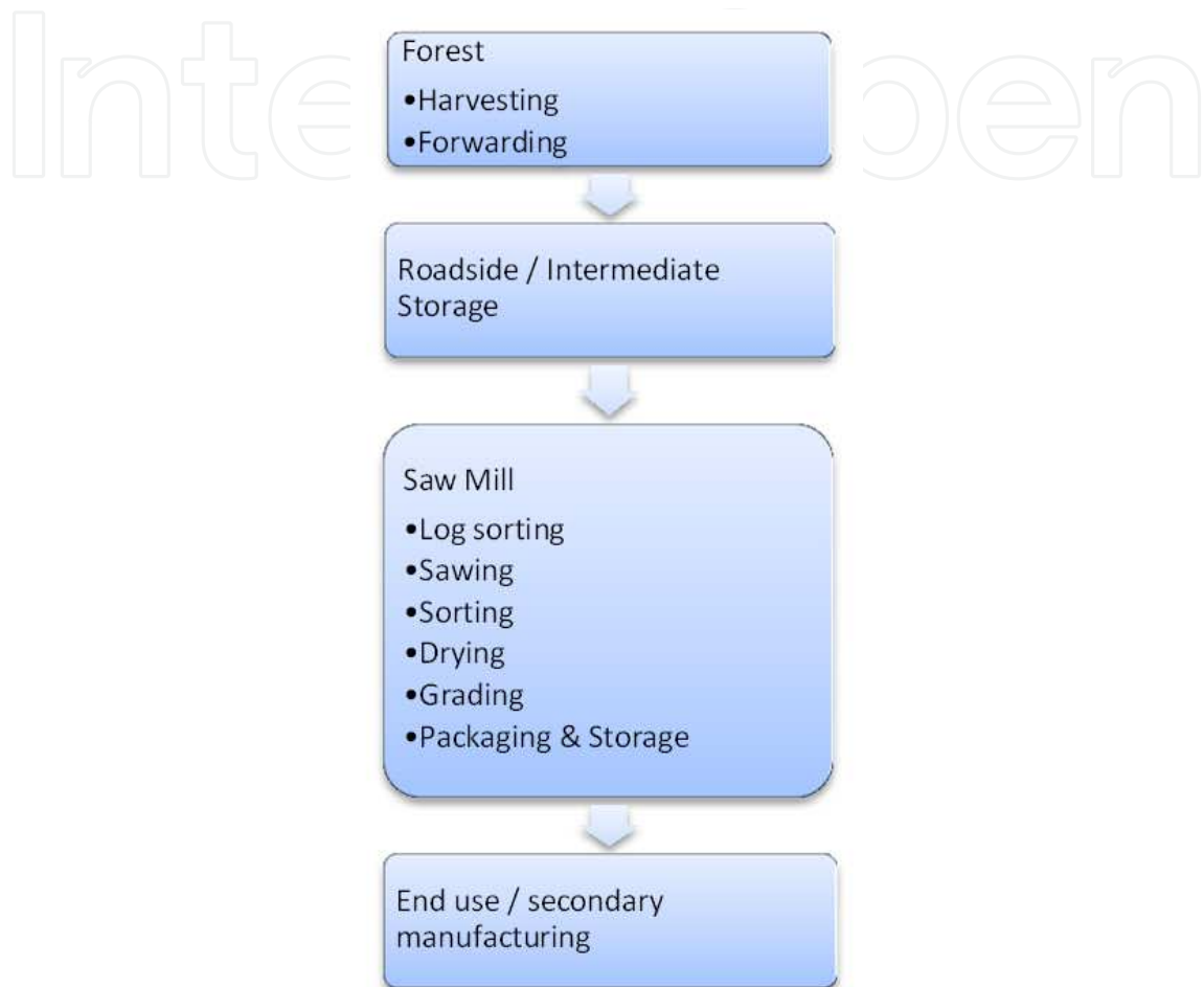
Figure 2. Nordic wood supply chain for sawn timber.
