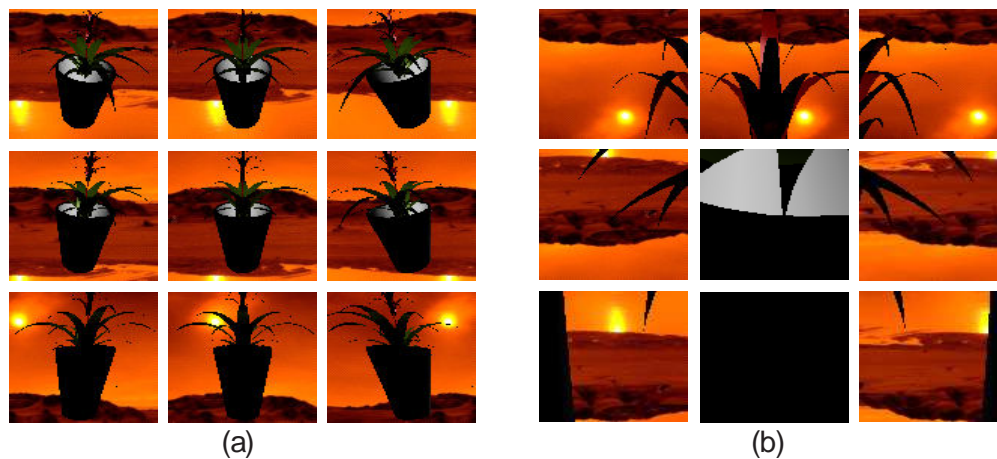
Figure 13. a) Perspective images from different views, (b) example of a hogel image.
