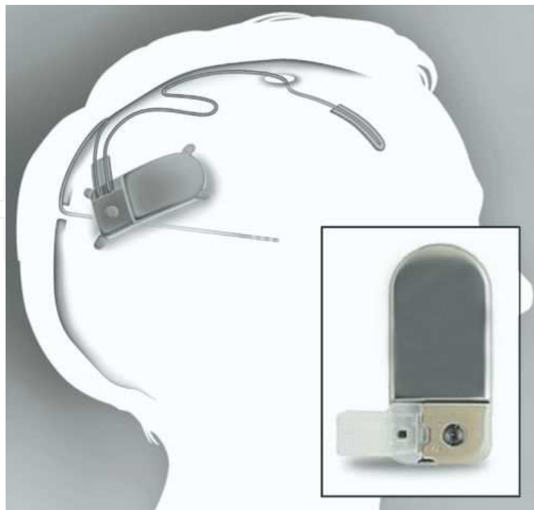
Figure 1. schematic graph of an implanted RNS stimulator, depth lead and cortical strip lead (NeuroPace, Mountain View, CA). The RNS neurostimulator (inset) has up to two leads. Either depth lead or cortical (subdural) strip lead is used in the system. Each has four electrode contacts that can be used for sensing and delivering stimulation. To obtain early seizure detection and delivery of focal electrical stimulation, leads are placed close to the seizure focus (Morrell et al, 2011).
