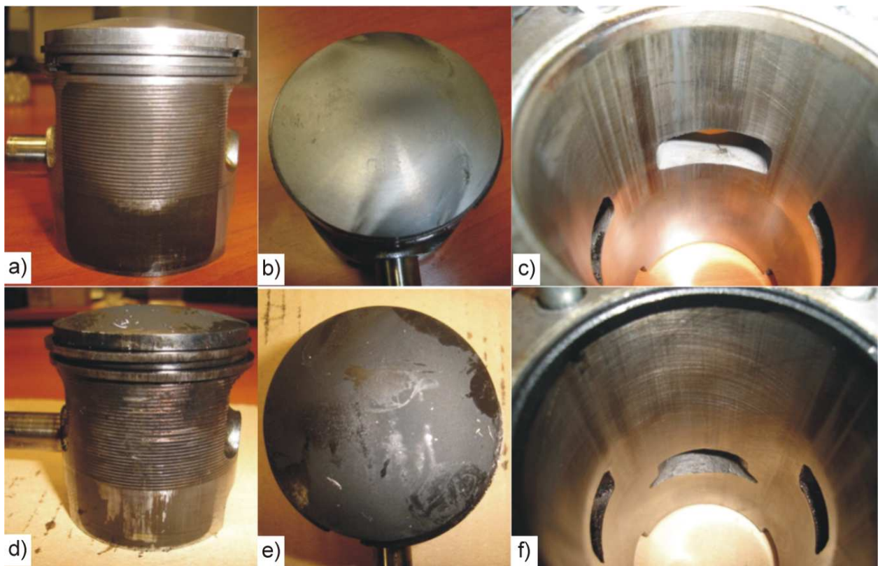
Figure 12. Macro images of two-stroke engine components after scuffing test using mixture of SEMO 36 lubricating oil with bioethanol E85 (a, b, c) and petrol (d, e, f): a), b), d), e) piston, c), f) cylinder in [12].
