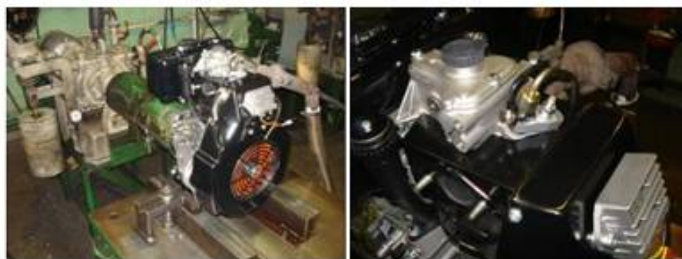
Figure 18. The engine on test bench and the tested nozzles installed on the engine
