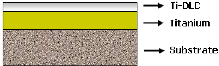
Figure 6. Scheme of titanium doped DLC coating. In this case, the first titanium layer was deposited in order to improve adhesion of DLC coating to the substrate and relax stress of the coating
