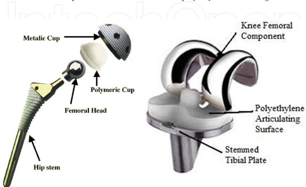
Figure 3. Schematic diagram of artificial hip joint (left) and knee implant [29] (right)
