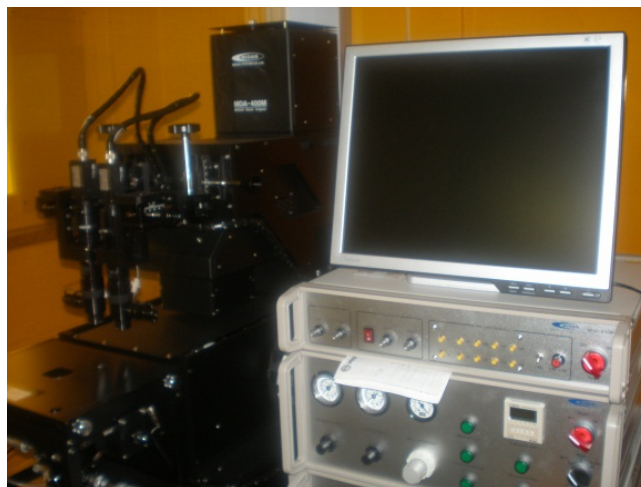
Figure 2. Mask aligner system (MDA-400 M) for lithography pattern fabrication
