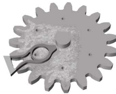
Figure 20. Schematic of the microengine affected by friction and wear
