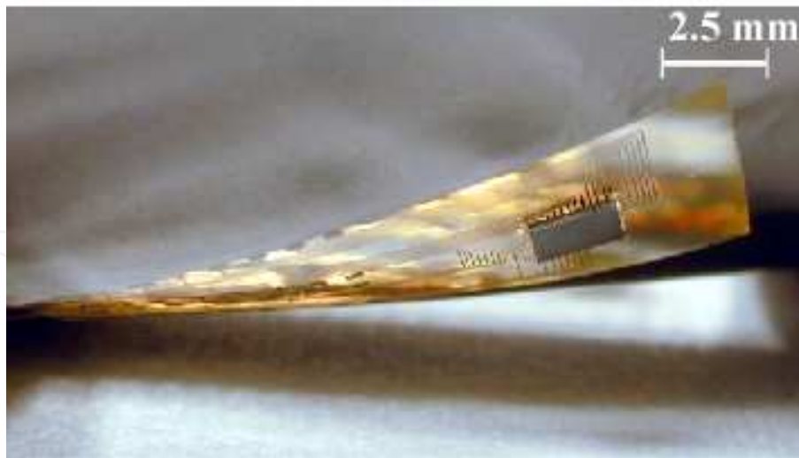
Figure 34. Demonstrates flexibility of CL-I 2 package. Chip can be seen underlying overlying parylene “skin.”
