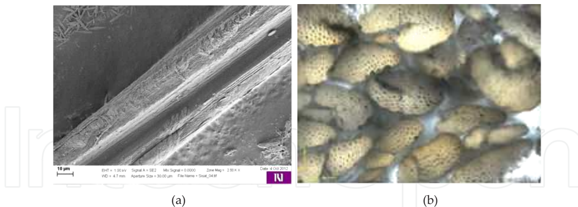
Figure 8. a) Longitudinal view (2500x magnification) and b) cross-section of sisal fibre
