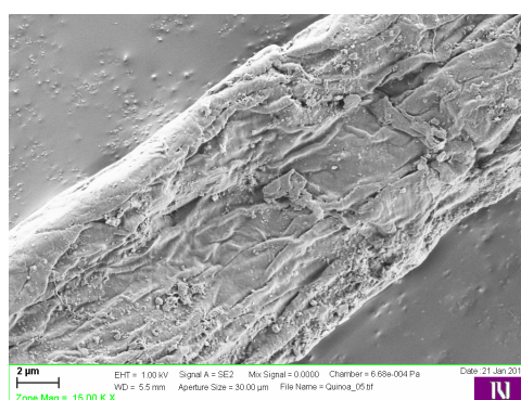
Figure 11. SEM image of surface morphology of isolated fibres from quinoa (fibres obtained by decortication from untreated stems)
