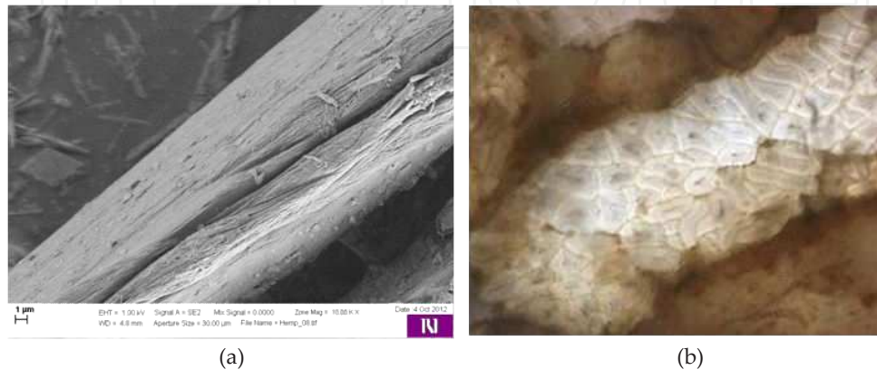
Figure 6. a) Longitudinal view (10000x magnification) and b) cross-section (200x magnification) of hemp fibre
