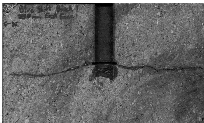
Figure 2. Example of serial sectioned hydraulic fracture showing growth from a notch in a 16 mm diameter wellbore.
