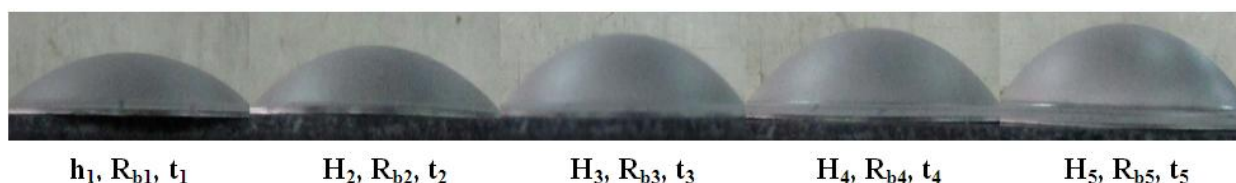
Figure 11. Photography of the bulged sample in stepwise approach
