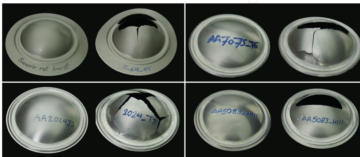
Figure 10. Burst and not burst samples of Ti-6Al-4V alloy
