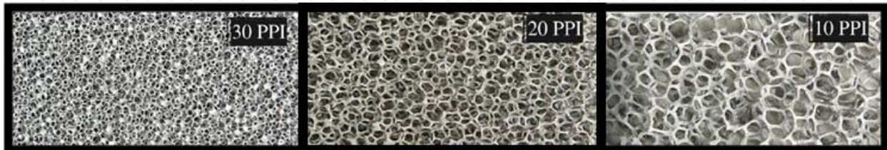
Figure 7. Metallic foam of different pores per inch.
