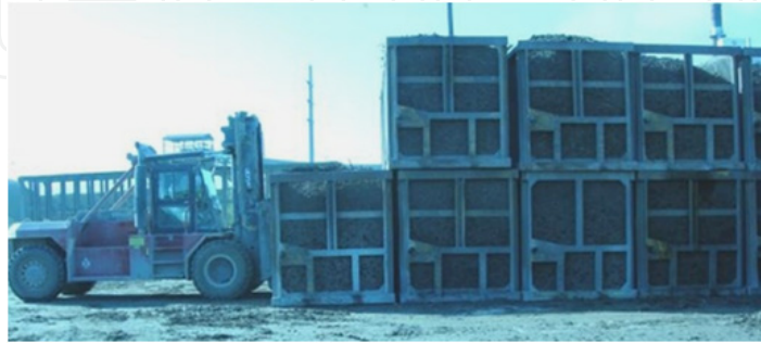
Figure 12. Bins being stacked in at-plant storage at sugar mill in South Florida, USA.
