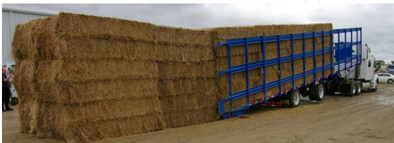
Figure 9. Self-loading trailer built by Kelderman Mfg. to implement multi-bale handling unit concept for 36-bale stack of large rectangular bales.
