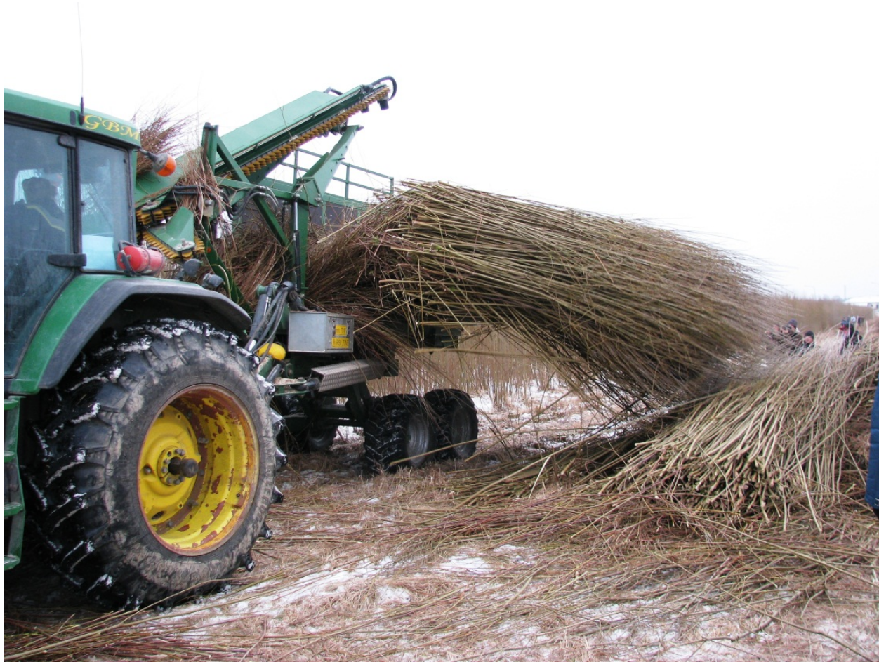
Figure 11. A tractor-pulled whole shoot harvester, unloading willow shoots at the headland (Photo: Nils-Erik Nordh).
