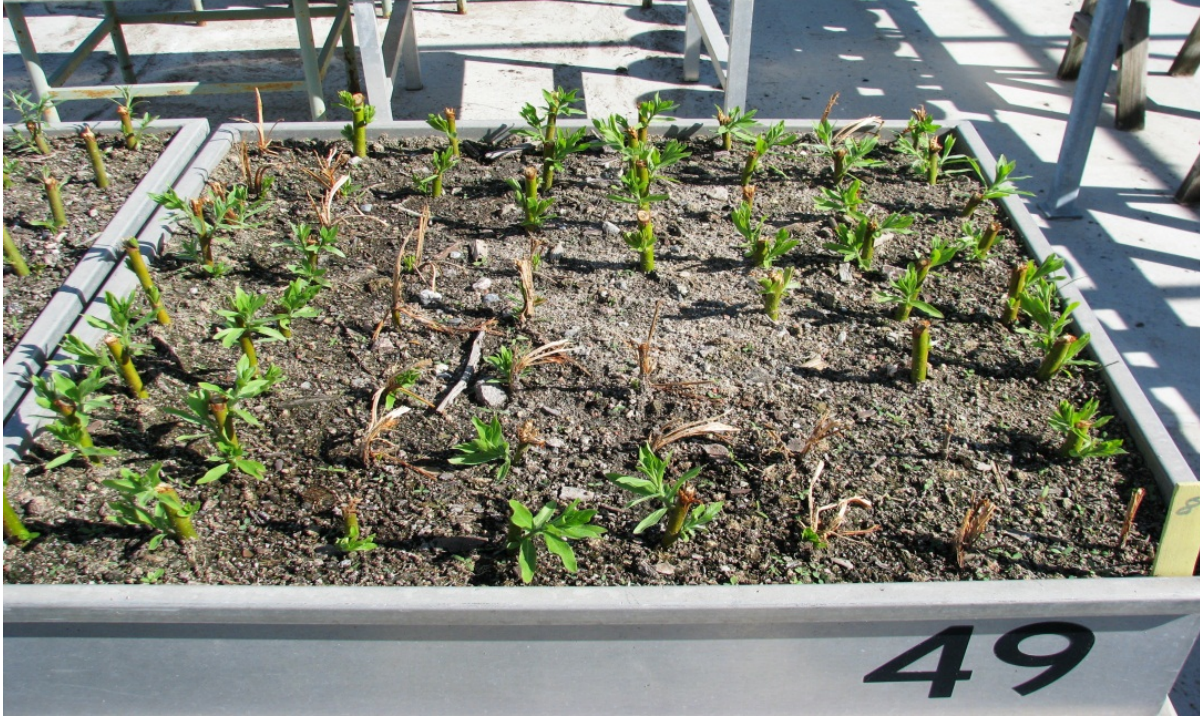
Figure 5. Cuttings planted by machine in a hard soil were transformed to a soft soil to isolate the effect of machine planting from other factors. The thinner cuttings were visually damaged and displayed a lower sprouting performance than the thicker ones (Photo: Nils-Erik Nordh).
