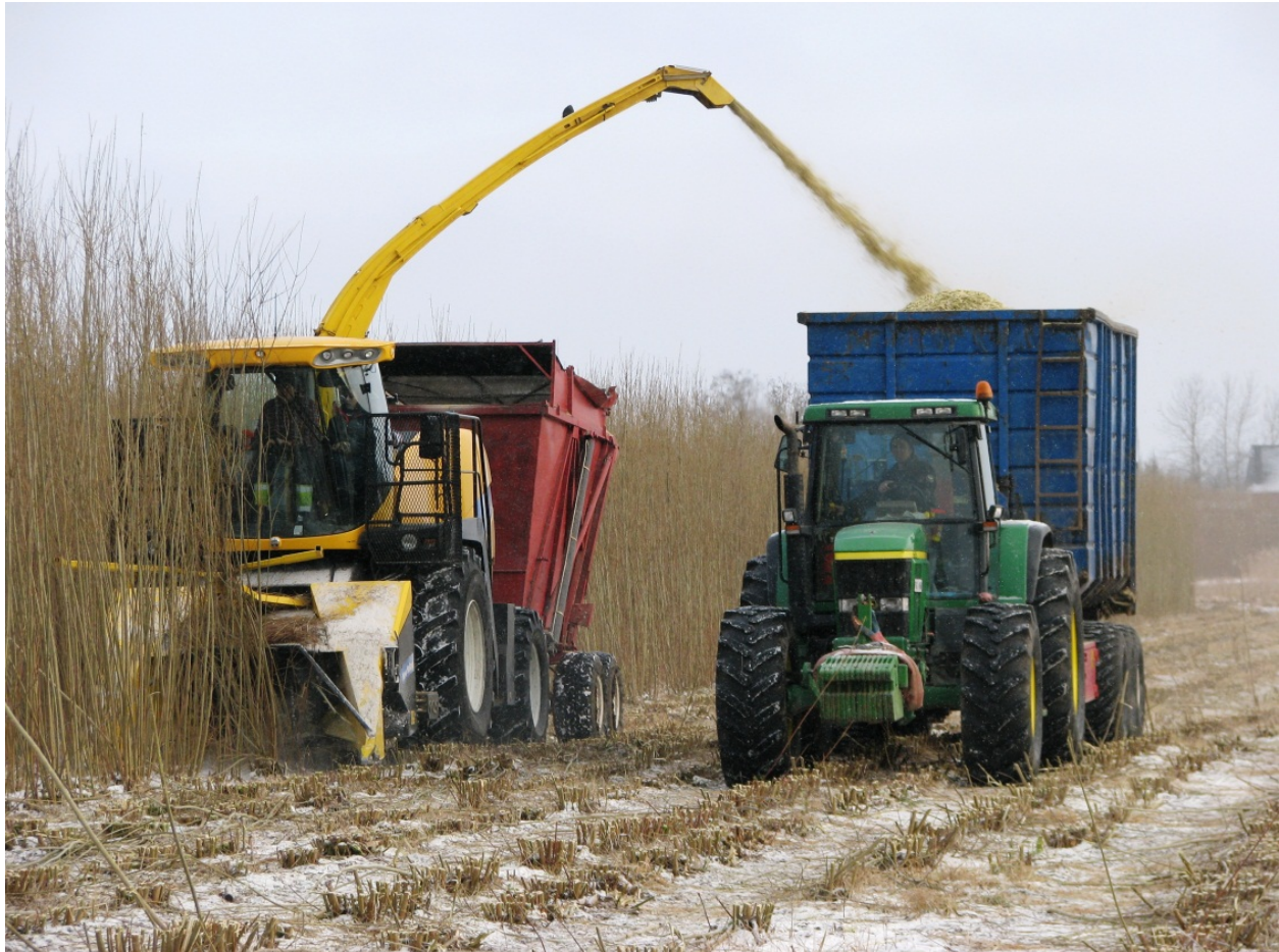
Figure 9. Willow harvest by means of a self-propelled chipper which blows the willow chips in an adjacent container (Photo: Nils-Erik Nordh).
