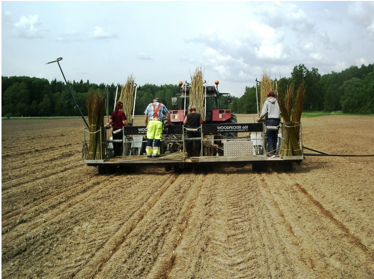
Figure 1. Machine planting of willow by means of a Woodpecker 601, using long rods and planting three double rows at a time (Photo: Nils-Erik Nordh).
