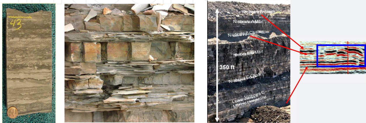
Figure 4. On every scale, formations may have laminations that hinder vertical permeability and fracture penetration. Shown are thin laminations in the Middle Bakken [11], layering in the Woodford [outcrop photo courtesy of Halliburton], and large scale laminations in the Niobrara [adapted from 12] [13]
