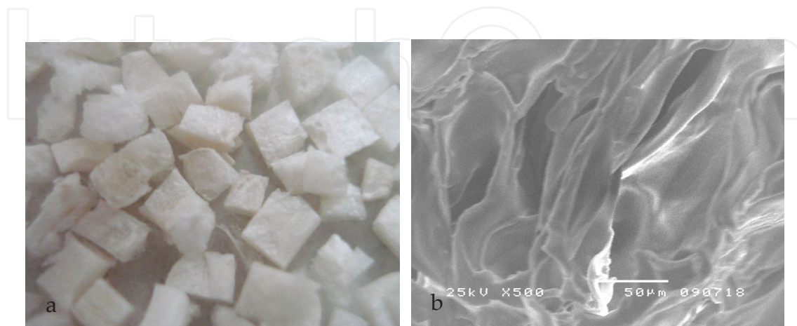
Figure 4. Gelatin-Alginate. Block (a), SEM (b)
