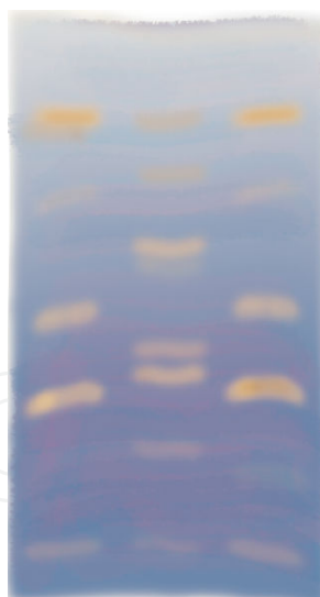
Figure 4. Compounds resolved on the TLC plate after spraying with DPPH methanolic solution.
