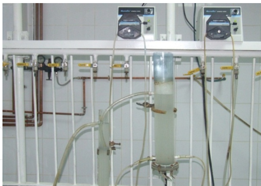
Figure 4. Laboratory simulation of aerobic sewage treatment
