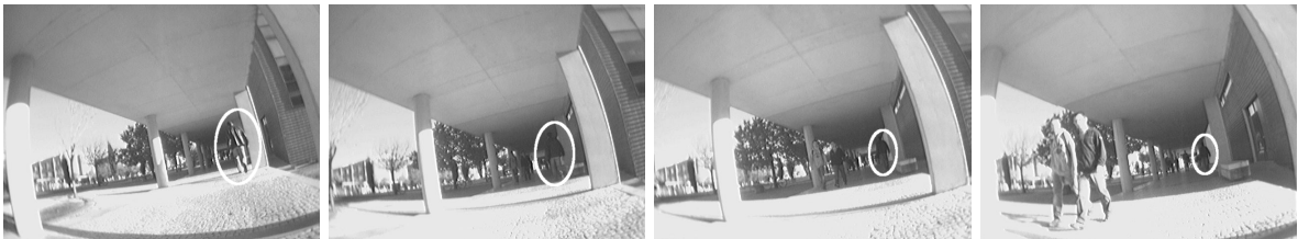
Figure 5.10: Bad leader: the subject marked with a white circle moves too fast compared to the robot's speed and gets too far from it.
