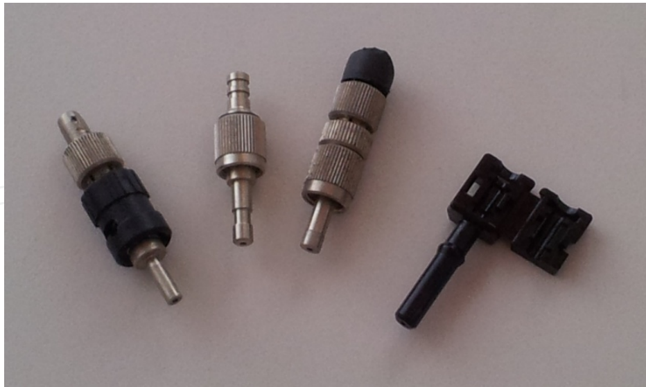
Figure 12. Different type of 1 mm POF connectors. ST, SMA (2 versions), V-pin. Other type of connectors exist.
