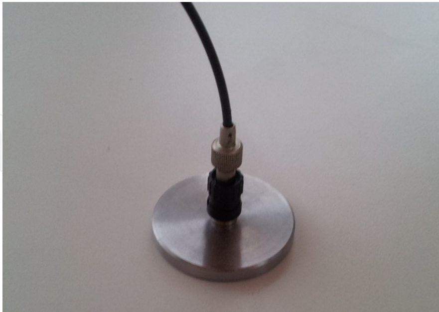
Figure 13. Polishing disk for 1 mm POF. This disk will be moved forming several times a 8-shape on sand paper for final cleaving.
