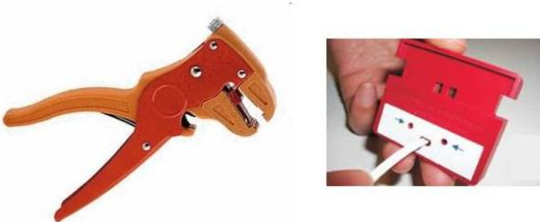
Figure 11. Cutting and stripping tools. On the left, a conventional copper cable stripper; on the right, a proper tool courtesy of Firecomms.
