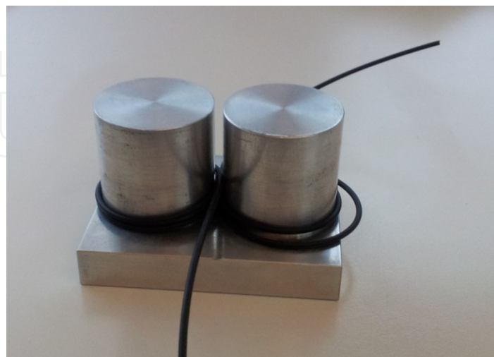
Figure 9. Mode scrambler. Two cylinders with a radius of 21 mm are separated by 3 mm. The fiber is wound in a 8-shape 10 times around those cylinders. The total attenuation of such an arrangement is about 10dB.
